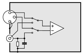
Essentially a differential input is a floating input. Nothing more, nothing less. The only reason why one should consider including an RC combination is to keep the signal within the common mode range of the input circuit (remember that the source may be floating) and to keep RFI that's been picked up by the RCA cable out of the box.
