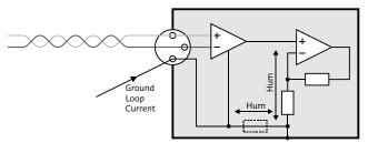
The root cause is the fact that an unthinkingly connected pin 1 functions as an unplanned input that gives direct access to an internal wire that nobody has any business with. This is completely unnecessary and counterproductive.
