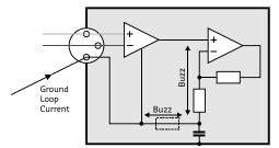
Now, a 500nF capacitor may be a high impedance at 50Hz, at 4kHz it's not. Hum with the fundamental and lower harmonics removed is called "buzz". It's hardly an improvement.
